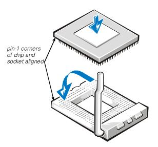
Figure 8-12. Installing the Microprocessor Chip
